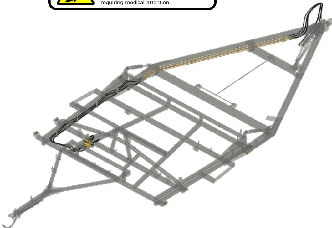
***Air Seeder Hydraulic Circuit – (shown with optional floating A-frame hitch)***
